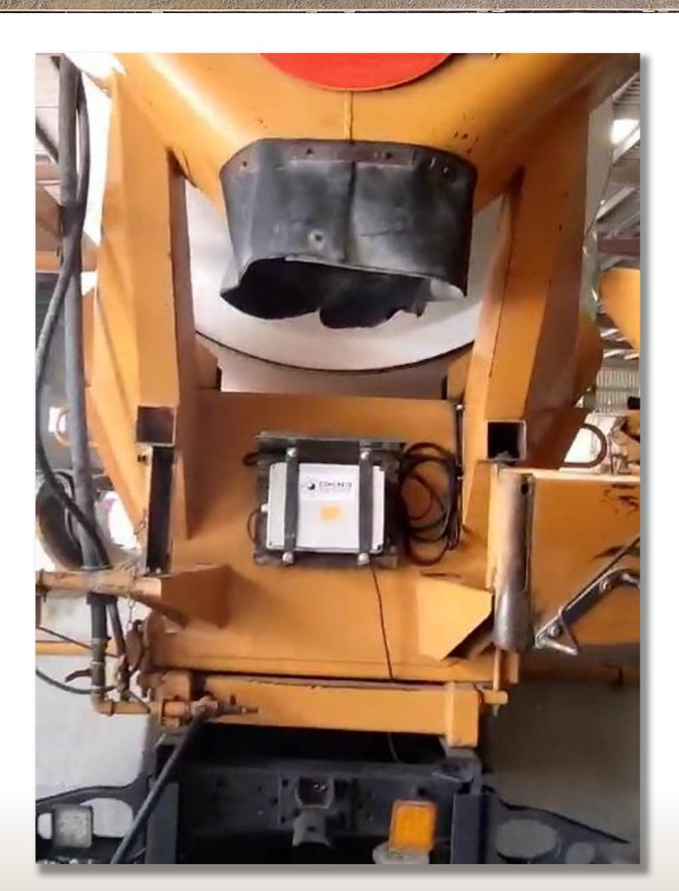
Standard position (below) alternative (left), fixed with welded stirrups.
