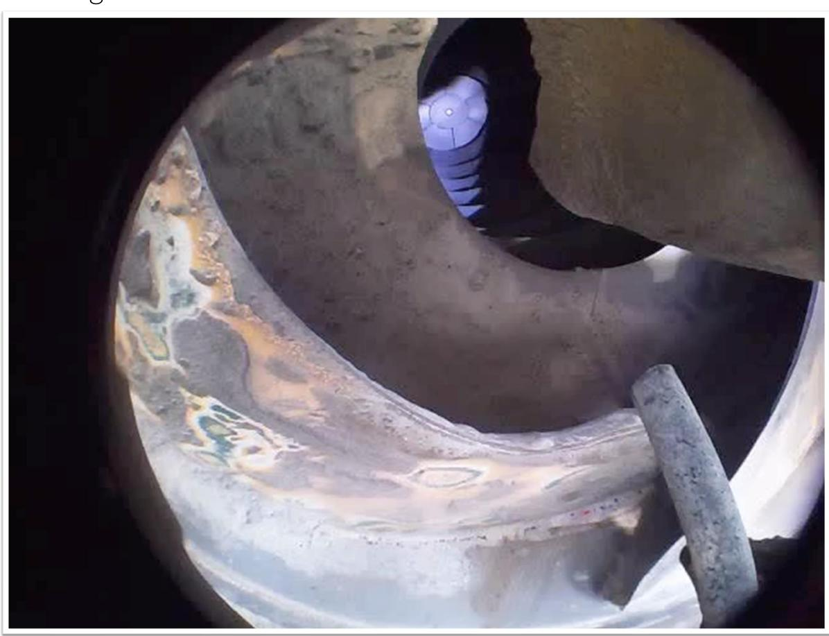
Drum rotating, notice down-right the water and admixture hoses. Observe water addition at 0:37 seconds.
